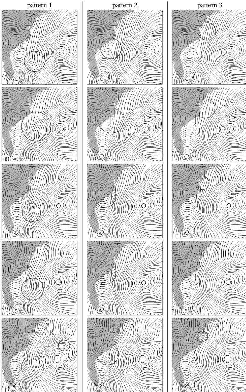
Figure 3: Interactive pattern recognition for the first five hours of a flow simulation (Hurricane Isabel at 3150 meters height): three patterns are selected from a slice at an early time step. The patterns, which stay similar, can be tracked over time.
