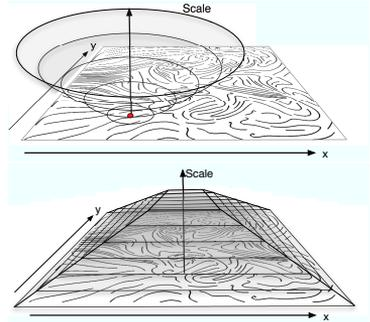
Figure 2: Illustration of a moment pyramid. Moments are computed for varying pattern sizes. Starting with a minimum pattern size of  $5 \times 5$  the moments are computed for the maximum possible pattern size (limited by the size of the flow field). Storing the moment values for each scale and position results in a pyramid structure.
