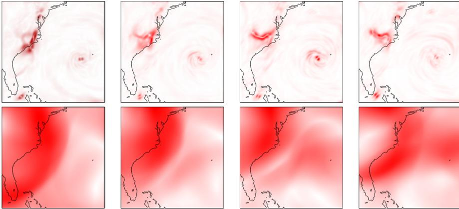
Figure 5: Moment pyramid comparison for different time steps of Hurricane Isabel. Distances on level one (high-frequency changes) are visualized in the upper row for similarity-distances between the time steps 1-2, 2-3, 3-4, and 4-5. In the row below, a higher level (half the pyramid’s height) distance is visualized for the same time steps (indicating low-frequency changes).
