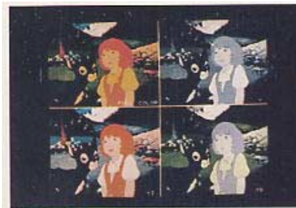
Figure 13: Full color RGB image digitally transformed into YIQ color space and retransformed back into RGB space using only Y, only YI, and only YQ.
