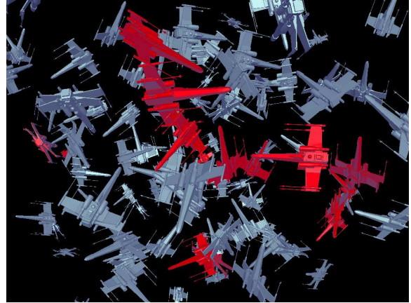
Figure 5: Example of a complex model scenario requiring kinetic sweep and prune, along with OBB-trees for efficiency. Each of the 100 models is composed of over 6000 triangles, for a total of over 600,000 triangles; our collision detection engine sustains over 15 frames per second, including dynamic intersection tests. Red models are colliding.
