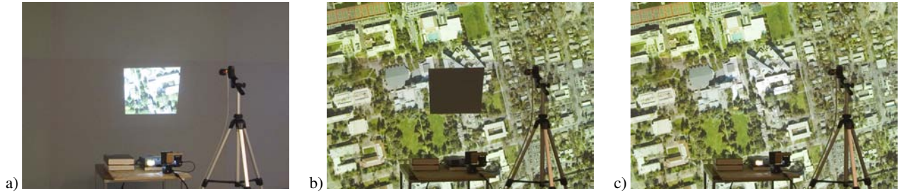
Figure 7: a: Projection of foveal inset only. b: Projection of main application onto display wall with foveal inset area masked. c: Final view combining rear projection and foveal-inset projection.
