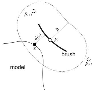
Figure 3: A brush at position  $p_i$  interacts with a model. Vertex  $x$  on the model’s surface is within the region of influence  $h$  of the brush. As the brush moves through space, the warp function transforms the surface vertices within the region.
